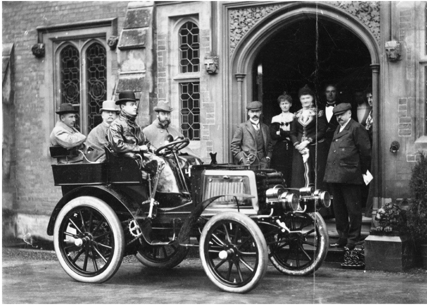
Above: The 1900 12 h.p. Panhard racer was rebodied in August 1900 as an aluminium rear-entrance tonneau painted in the Llangattock colours of dark green lined yellow. Rolls is at the wheel with the Duke of York, later King George V in the passenger's seat. Rolls's father Lord Llangattock is in the rear behind the Duke with Sir Charles Cust, the Duke's equerry. Lady Llangattock is standing at the entrance to The Hendre in the centre.
