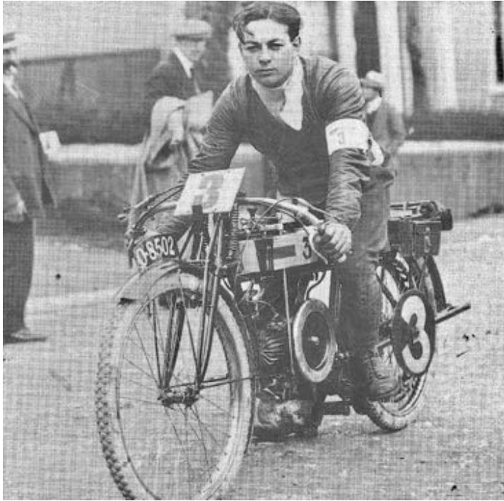
Above: Les Bailey and the 2¾ h.p. Douglas on which he set the record of 70 m.p.h. for the 350 c.c. class at Brooklands. [‘Motor Cycling’ 24 December 1912]
